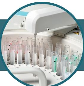
**Integrated HbA1c hemolysis: practical and agile.** Throughput of up to 626 tests/hour, with STAT priority loading. Features dedicated probes, an independent mixer, and automated HbA1c hemolysate preparation to reduce errors and optimize workflow.
