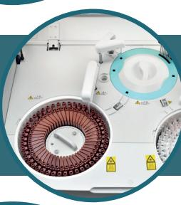
**Low reaction volume and low cost per test.** Requires only 90 µL per reaction, optimizing reagent efficiency. The dry bath system minimizes routine maintenance and consumes less than 20 L/h, with an efficient wash system to prevent cross-contamination.
