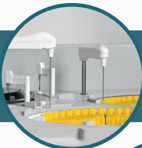
**Productivity and Flexibility.** Nominal speed of 600 photometric tests/hour; 1000 tests/hour when combined with ISE (optional). Featuring 12 refrigerated positions for reagents. Barcode reader for samples and reagents, speeding up laboratory routine.
