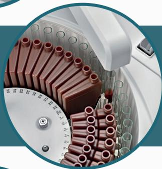
**High capacity of on-board reagents.** High capacity of simultaneous reagents in tray: Up to 100 interchangeable positions of reagents, granting more autonomy to routine execution. 20 mL or 40 mL reagent vials. Detection of vertical obstruction and level monitoring of sample and reagent.
