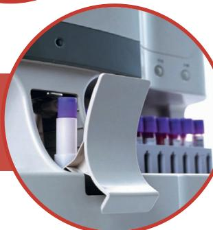
**High productivity and dynamism.** Low consumption of reagents, speed of up to 60 samples per hour with possibility of insertion of an emergency sample with automatic loading.
