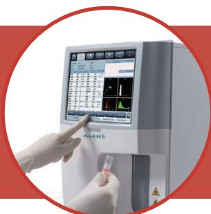
**High productivity and cutting-edge technology.** A differential 5-part analyzer, measurement of 25 parameters, 4 research parameters, histograms and 1 scatter plot of blood samples. Electrical impedance to determine RBC and PLT. Laser flow cytometry and calorimetry for hemoglobin determination with reagents free of cyanide, with no risk to the environment.
