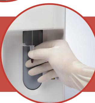
**Low consumption of sample and higher economy.** It uses a reduced volume of sample, minimizing re-collections and offering the best performance. It uses a 15 µL sample in whole blood mode and 20 µL in pre-diluted mode. Ratio of dilution in pre-diluted mode superior to other analyzers of the same size, promoting an excellent performance.
