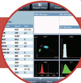
**Complete, simple and intuitive software.** Featuring a 10.4 inches touch screen, bringing practicality to users and no need of an external computer. It automatically stores up to 40,000 records. Evaluation of controls by Levey-Jennings Charts, simplifying CIQ management.
